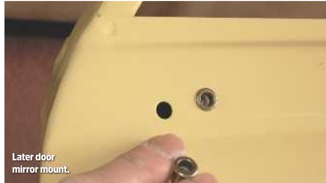
Early 1970's passenger door, drilled for dealer supplied (Unipart) mirror.
