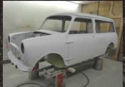
After being etch-primed in the VVCR paint booth.
