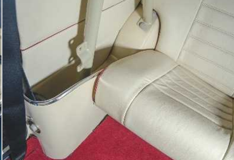
Above: The Mk2's two-part headlining frame has been retrimmed with cream suede. Even the rear companion bins have been covered in matching cream leather. Below: Both the slightly modified Rover top dash rail and custom bottom dash rail were changed from the grey leather to the cream hide. Newton Commercial red carpet lifts the interior nicely and the wood steering wheel, dash and gearknob add a touch of luxury. Note the custom switch panel and screen in glovebox.
