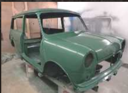
The repaired bodyshell was painted in two-pack Almond Green paint and then flatted back.
