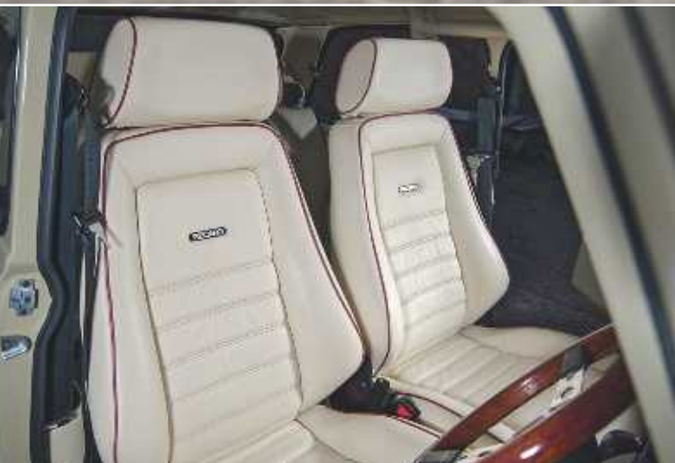
Above: The supportive Recaro reclining front seats, which were originally fitted to this Mk2 when it was first restored, look way cooler now they have been retrimmed in cream leather with contrasting red piping. And there is even a matching rear bench seat. The rear headrests have been bolted to the rear bulkhead.
