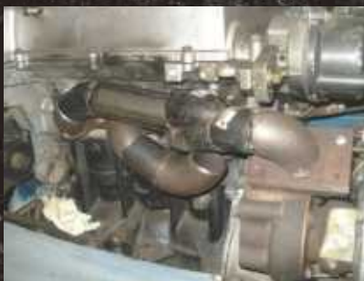
Ben undertook the super-compact exhaust manifold with turbo flange. Tiny Garrett hybrid is just above the gearbox. You can see repositioned alternator near to block coolant inlet elbow.
