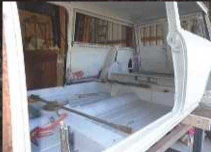
An M-Machine replacement floorpan was fitted.
