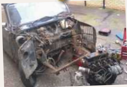
Front end was rotten
