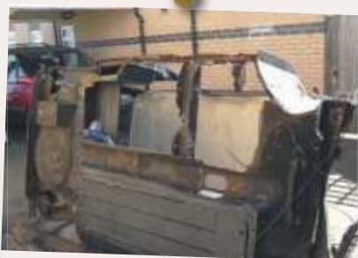
Cutting out more rust
