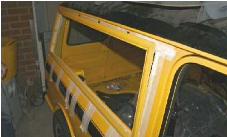
Loads of masking tape was needed in order to protect the paint when offering up the frames. With the bottom holes lined up we could firstly clip the top rail in position and then push the bolts in the bottom rail through the bodywork before securing them with the tiny nuts.
