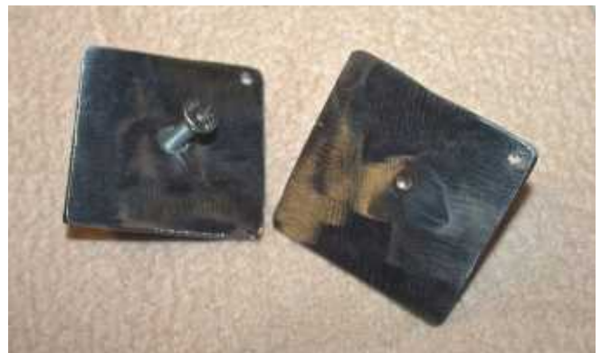
I have made six small spreader plates, each with an M5 stainless screw, with the underside ground back. Once painted these were bonded to the upper edge of the inner wing and I will secure the loom to them, using P-Clips.
