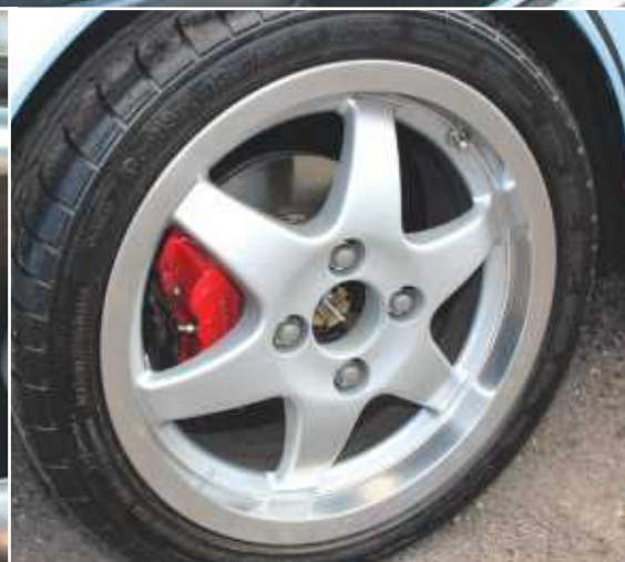
Wheel stud upgrade to 7/16-inch goes hand in hand with PCD change to 100mm. Diameter overall is very close to (19.6-inch) Sports Pack, despite 14-inch alloy wheels.
