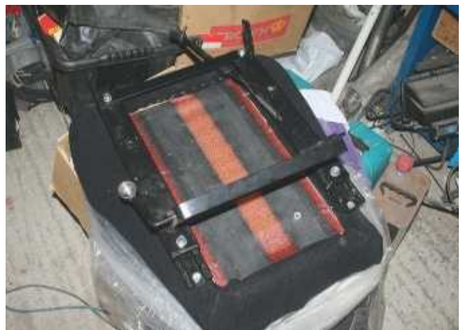
The customised Corbeau Classic bucket seats came with Mini-specific frames to secure to the OE brackets, which are mounted on the crossmember.
