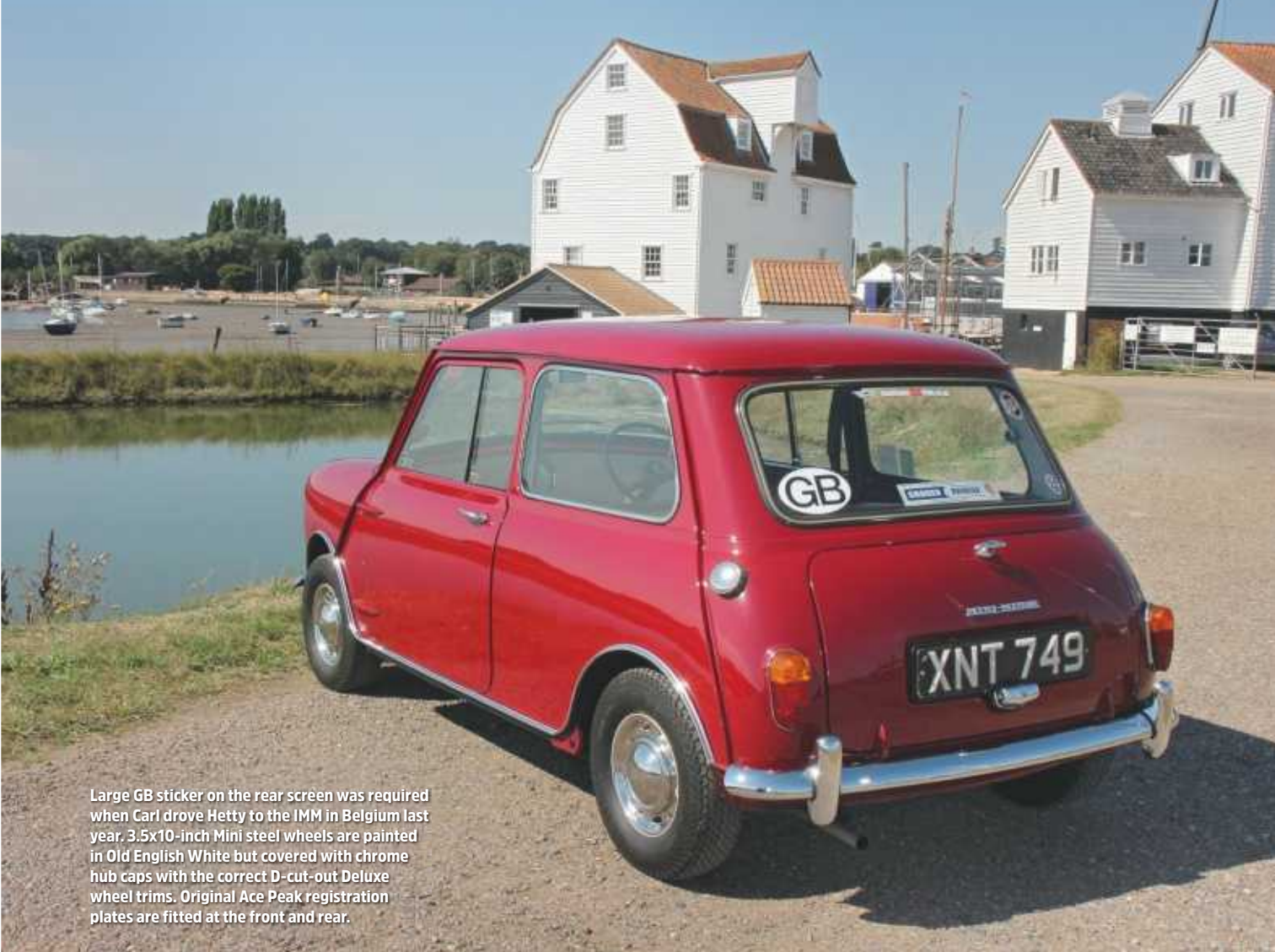
Black plastic mouldings on the kick plates were fitted to early Morris Minis.
