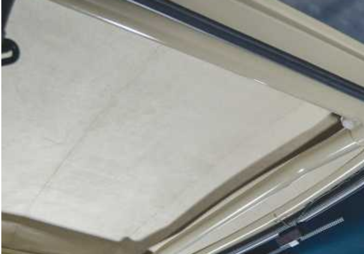
Above: The Mk2's two-part headlining frame has been retrimmed with cream suede. Even the rear companion bins have been covered in matching cream leather. Below: Both the slightly modified Rover top dash rail and custom bottom dash rail were changed from the grey leather to the cream hide. Newton Commercial red carpet lifts the interior nicely and the wood steering wheel, dash and gearknob add a touch of luxury. Note the custom switch panel and screen in glovebox.
