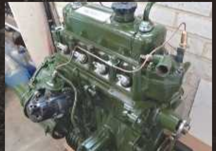
Back from Mini Speed, after the rebuild, and fitted with a replacement 12G202 cylinder head.
