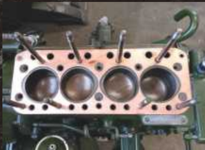
With the cylinder head removed the 998cc engine's MOWOG pistons are visible.
