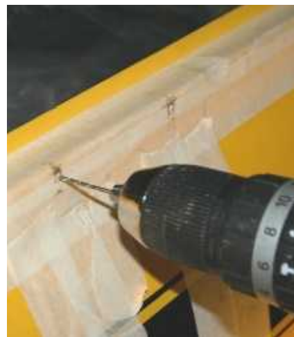
This was certainly a case of measuring once, twice, having a brew and measuring again, before drilling. The M-Machine side panels don't come pre-drilled and, when the shell was painted we didn't have any usable frames, which wasn't ideal.
