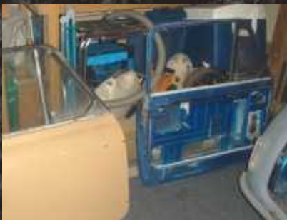
You don't see these very often in the UK and that's a big shame. These are Aussie-spec external hinged doors with steel pocket, wind-up glass and hinged front quarterlight. A crafty design.
