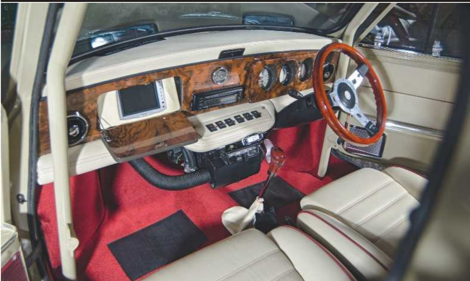
Above: The Mk2's two-part headlining frame has been retrimmed with cream suede. Even the rear companion bins have been covered in matching cream leather. Below: Both the slightly modified Rover top dash rail and custom bottom dash rail were changed from the grey leather to the cream hide. Newton Commercial red carpet lifts the interior nicely and the wood steering wheel, dash and gearknob add a touch of luxury. Note the custom switch panel and screen in glovebox.
