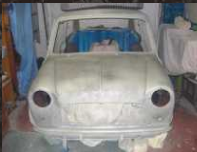
Mini K shell undergoes paint prep in Brad and Jodie's garage. With some modification of the front panel the clever and reliable Daihatsu three-cylinder engine fits the round-nose Mini front end.
