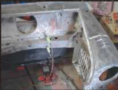
This Mini K bodyshell might have been white originally. The steel was amazingly good for the A$1000 price but the same model would cost a lot more today. Note fuel flow and return pipes.
