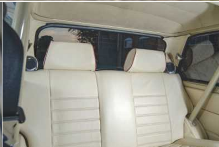
Above: The supportive Recaro reclining front seats, which were originally fitted to this Mk2 when it was first restored, look way cooler now they have been retrimmed in cream leather with contrasting red piping. And there is even a matching rear bench seat. The rear headrests have been bolted to the rear bulkhead.
