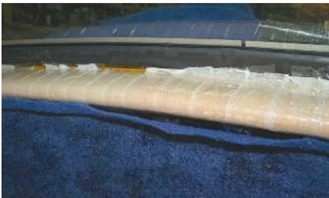
...but, disappointingly, it didn't stop the resin impregnated fleece from shrinking back. It has curved exactly as I wanted it but is too small. It may be a good starting point for another go but I will try another option first.
