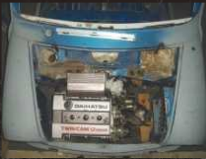
A cunning plan... GTi mill, minus turbo here, sits inside Mini K engine bay. Three-cylinder block is compact and not tall, as gearbox sticks out of the nearside. Front to rear clearance is a bit tight.
