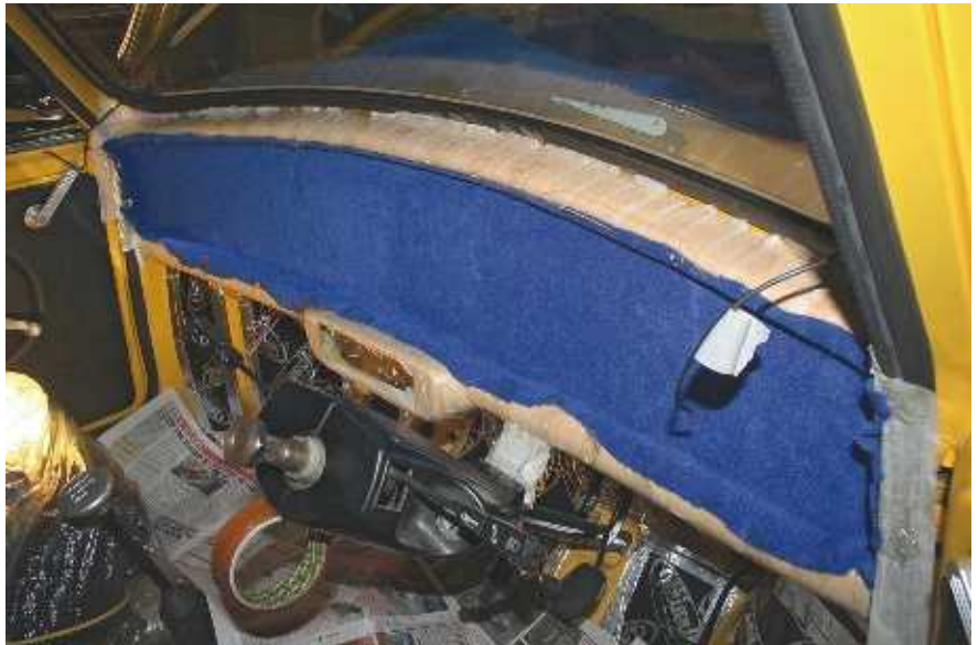
I covered the floor with newspaper and, with both of the dash rails protected with masking tape and Sellotape, the fleece fabric was then held in place using enough tape to supply Santa for a year...
