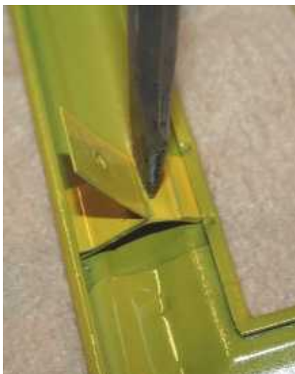
The side (C- and B-pillar) brackets are easier to work with. Some I had to replace and, once painted, I could press them back into place.
