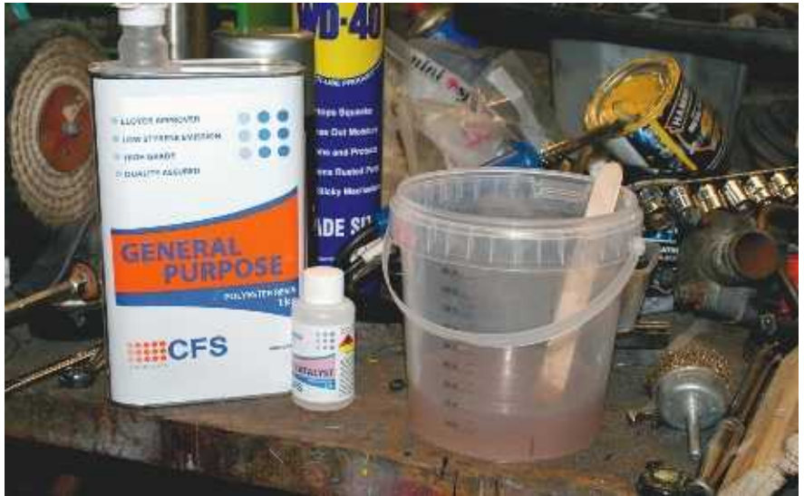
CFS supplied this easy to use general-purpose fibreglass resin. I find that using a liquid hardener, instead of a paste, as some companies sell, allows you to easily mix the two liquids and crack on with the job.
